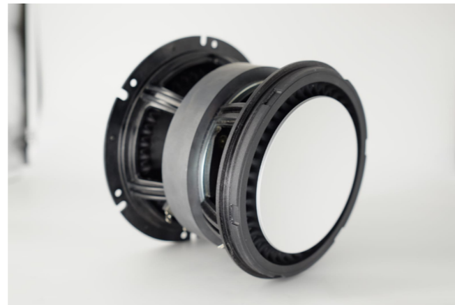
Figure 6. One of the two Uni-Core LF units found in LS60 Wireless
